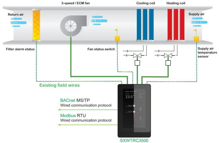
Low-Voltage Fan Coil Controller
